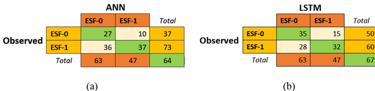
Fig. 14 Confusion matrix of the (a) ANN and (b) LSTM models on the daily ESF prediction. The top and right panels, respectively, represent the model and observation based on the classification of two desired classes. Inside panels with two left diagonal green boxes represent the numbers of the correct prediction against observed values for both ESF-0 and ESF-1 classes. The two right diagonal green boxes represent the false prediction for both classes. The bottom green box is the total number of correct predictions of both classes. The two bottom orange boxes represent the total number of false and correct predictions of the model, and the right gold boxes are also the total number for the observation
