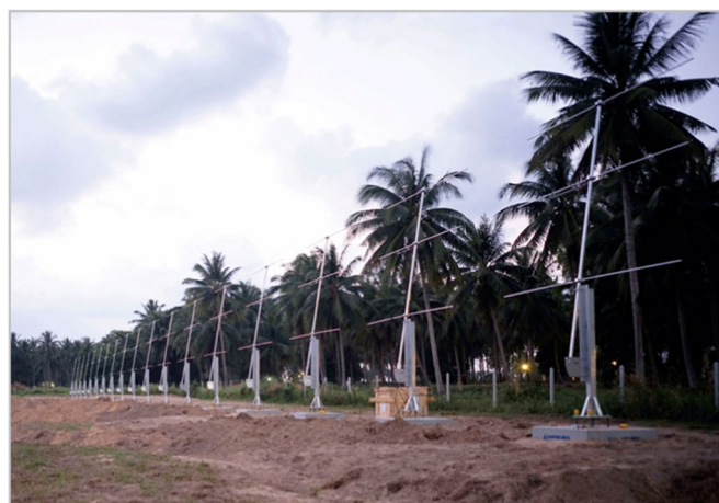
(b) VHF radar system for monitoring plasma bubbles
