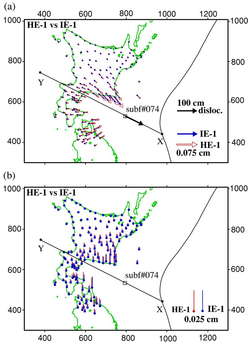
Fig. 5. Comparison of the surface displacements between homogeneous model HE-1 and inhomogeneous model IE-1. (a) Horizontal displacement vectors, and (b) vertical displacements. These figures show the surface displacements due to the reverse type dislocation of 1 m imposed on the cell-like subfault indicated in each figure. The line X–Y in each figure is that along which the surface displacement profiles are shown in Figs. 6(a), (b) and (c).
