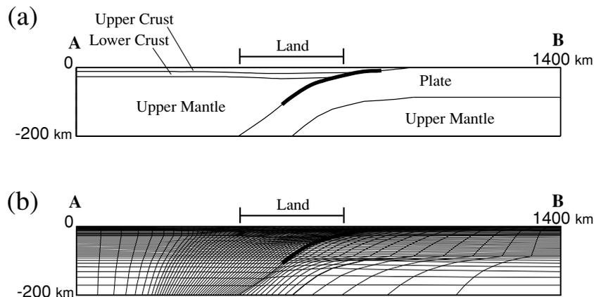
Fig. 4. Examples of vertical cross-sectional views (in  $\sim$ EW direction) for (a) subsurface structure and (b) finite element grid. These figures correspond to the line A–B in Fig. 3(a), and the thick lines along the Pacific plate interface indicate the portion on which the dislocations are imposed.
