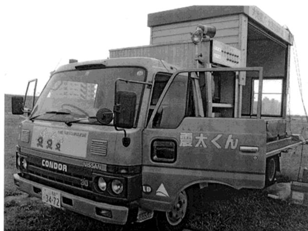
Fig. 2. Earthquake shake-simulator truck used in the UNSW-MRI GPS Seismometer Experiment.
