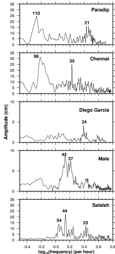
Fig. 4. Spectral analysis (FFT) of the detided water level records. The abscissa is  $\log_{10}(\text{frequency})$  (per hour) and the ordinate is the amplitude (cm). The period corresponding to the prominent peaks is shown by the numbers (in minutes).
