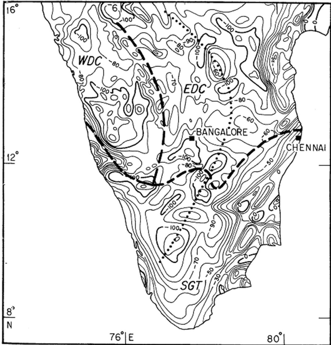
Fig. 8. Bouguer gravity anomaly map of India (Scale 1:5000,000) (NGRI, 1975). Possible extension of gravity trends from SGT to EDC is shown by solid dotted line.
