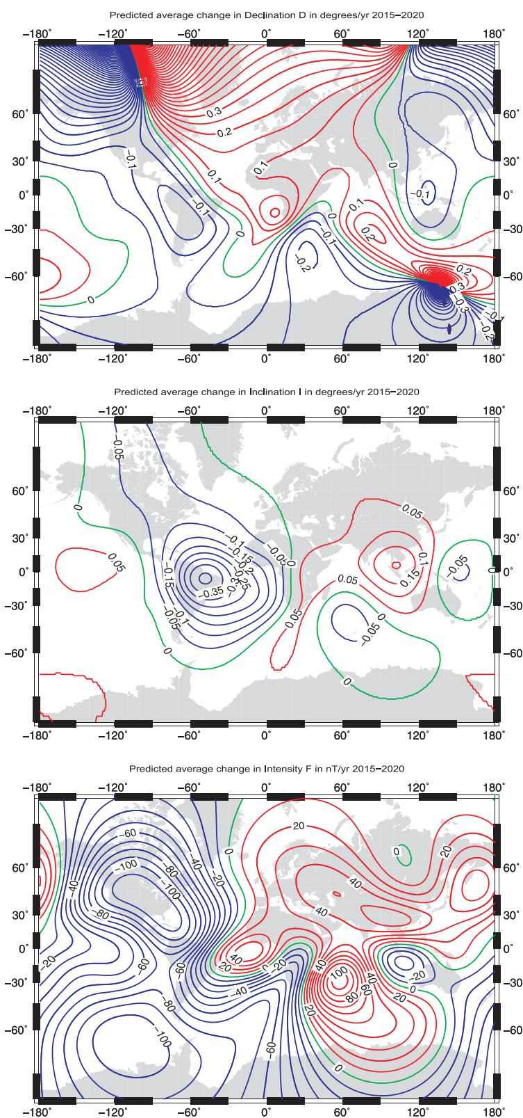
**Figure 2** Maps of the predicted rate of change per year in the declination D (top, units are degrees/year), the inclination I (middle, units are degrees/year), and total intensity F (bottom, units are nT/year) at the Earth's mean radius  $r = a$  for the interval 2015.0 to 2020.0. Projection is Mercator.
