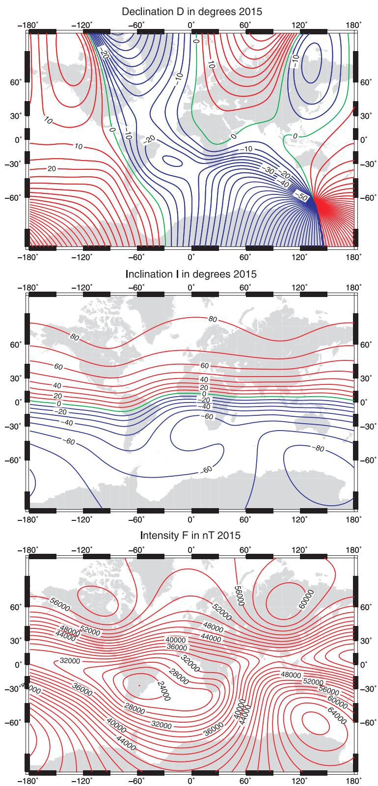
**Figure 1** Maps of the magnetic declination D (top, units are degrees), inclination I (middle, units are degrees), and total intensity F (bottom, units are nT) at the Earth's mean radius  $r = a$  in 2015; the red dot indicates the minimum intensity. Projection is Mercator.
