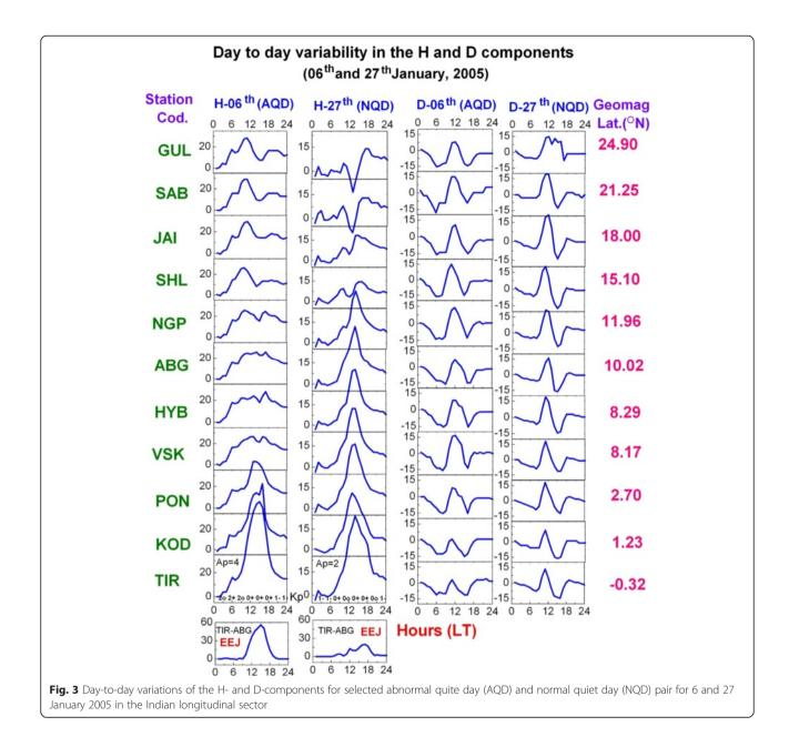
vortex during both the normal and abnormal quiet days is located near GUL (24.9°N geomagnetic latitude) for the stations situated along 75° E longitude.
