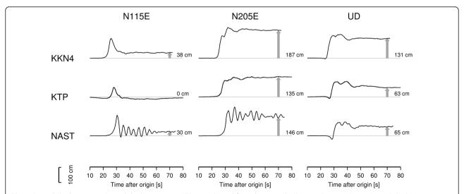
**Fig. 5** Ground displacements. Ground displacements at KTP were derived from the ground velocities shown in Fig. 3. Ground displacements at KKN4 and NAST were obtained by high-rate GPS records; these were downloaded from the UNAVCO website (Galetzka et al. 2015). The numbers attached to the *gray*, *bolded-arrows* indicate the amount of permanent deformation
