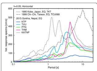
**Fig. 6** Horizontal velocity response spectra. The horizontal velocity response spectra for five sites in the Kathmandu Valley and two notable sites (TCU068 and TKT); these horizontal response spectra were obtained based on the maximum of the vector sum of the two horizontal-component response histories for a specific natural period by using the damping factor h = 0.05. The TCU068 and TKT records were downloaded from CESMD
