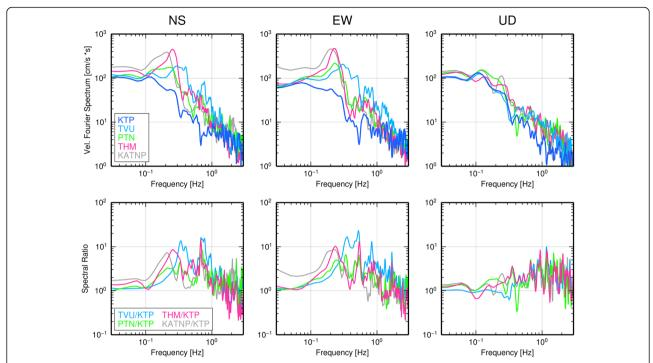
**Fig. 4** Fourier amplitude spectra and spectral ratios. The Fourier amplitude spectra of the ground velocities shown in Fig. 3 (*upper panel*). The ratios of amplitude spectra at the sedimentary sites to those at station KTP (*lower panel*)
