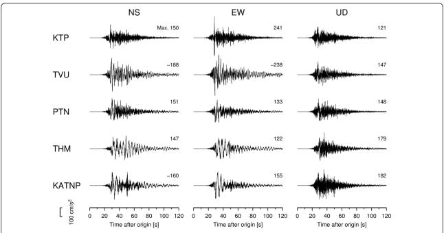
Fig. 2 Observed ground accelerations at five stations. These have been corrected for the sensor-response; KTP is a rock site and the others are soft sedimentary sites. The waveform records at KATNP were provided by USGS (2015b)
