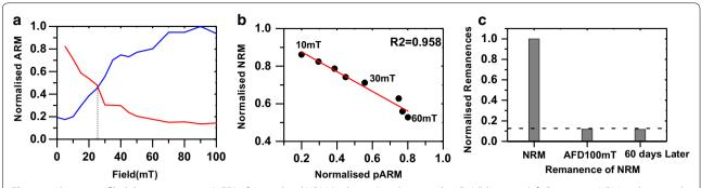
Fig. 7 a Alternating filed demagnetization (AFD) of normalized NRM (red curve) and acquired pARM (blue curve). b Remaining NRM and acquired ARM at the same applied field. c AFD remanences of the NRM and the variation of remanence over time
