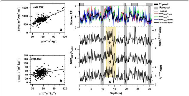
Fig. 6 Relative paleointensity (RPI) curves related to three magnetic concentration parameters. **a**, **b** Binary analysis of magnetic concentration parameters used in the RPI acquisition. **c**-**e** RPI curves obtained with different normalizers. **f** Stacked RPI in the BYH section. Gray bars highlight the RPI lows
