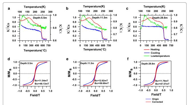
Fig. 2 a–c κ–T curves of representative samples (green line indicates the low-temperature susceptibility, while red and blues lines represent heating and cooling runs, respectively); d–f hysteresis loops of the same samples (blue lines are original data, and red lines are obtained after slope correction)
