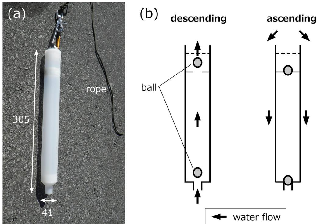
**Fig. 3** Photograph and schematic illustrations of the water sampling bottle. **a** Photograph of the water sampling bottle, and **b** schematic illustrations of the bottle. Numbers in panel **a** represent dimensions in millimeters
