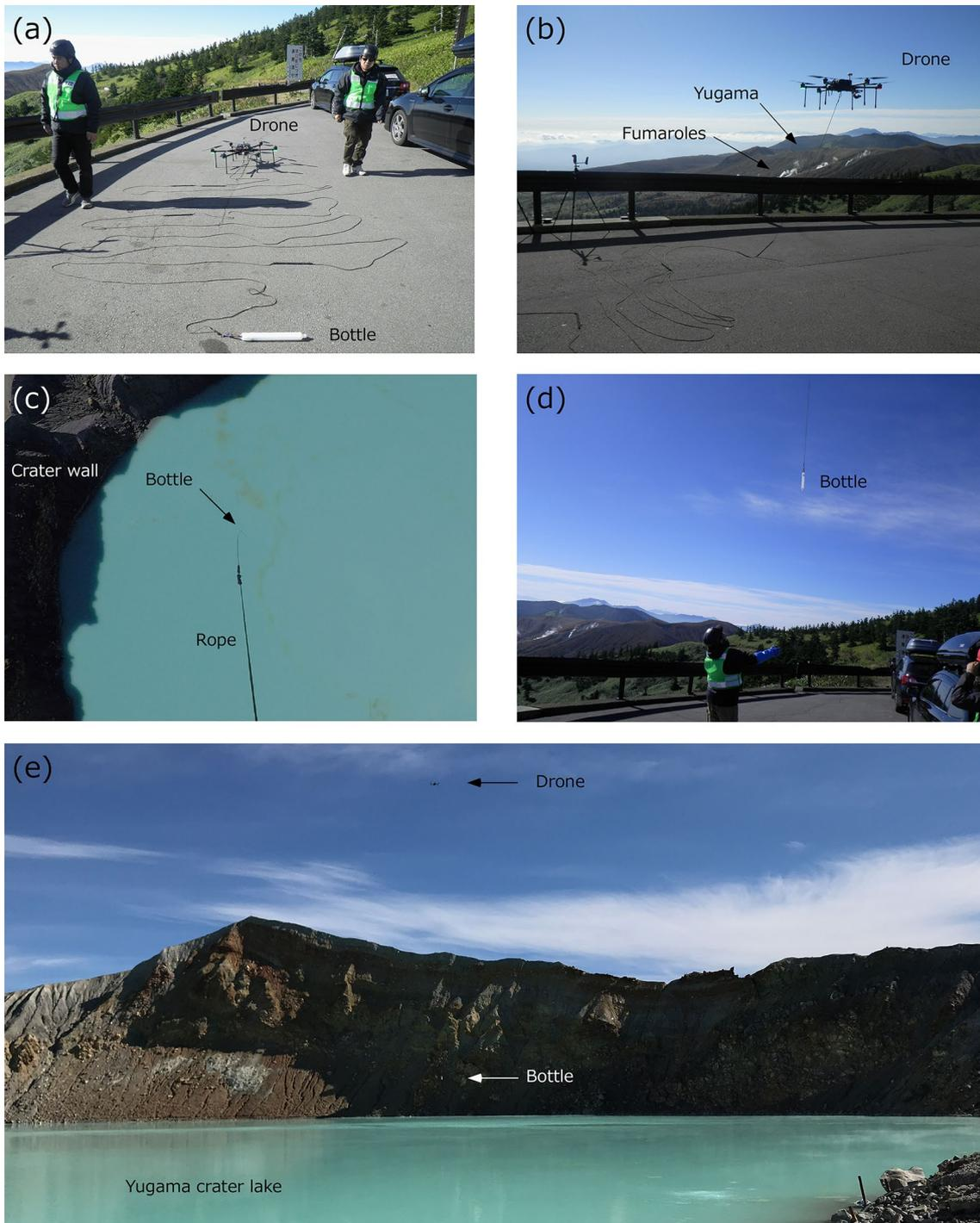
**Fig. 2** Photographs of the drone operation on October 18, 2017. **a** Setup of the drone LAB645, with the rope and sampling bottle on the ground. **b** Taking off with the suspended sampling bottle. **c** Photograph above sampling point B shown in Fig. 1, taken by a camera on the drone. **d** Catching the bottle by hand just before landing. **e** Approach of the drone and sampling bottle to the surface of Yugama crater lake
