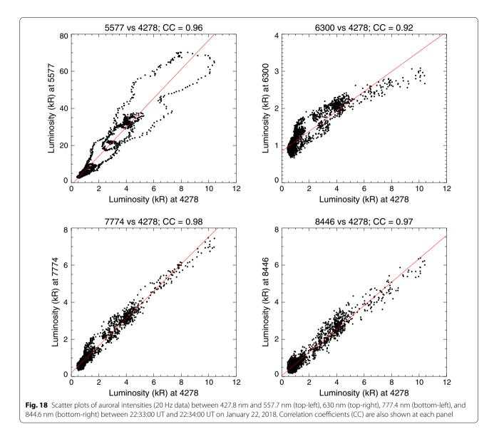
of the 630 nm emission. On January 22, 2018, two single events occurred, and on February 18, a single event occurred. For the 2 nights, the good linear relation is found, and the correlation coefficients are high, indicating the two emissions are well correlated even for an isolated event (i.e., single event). To conclude this, a cause of the swift rise of 630 nm is still unclear. To confirm a possible contamination effect in more
