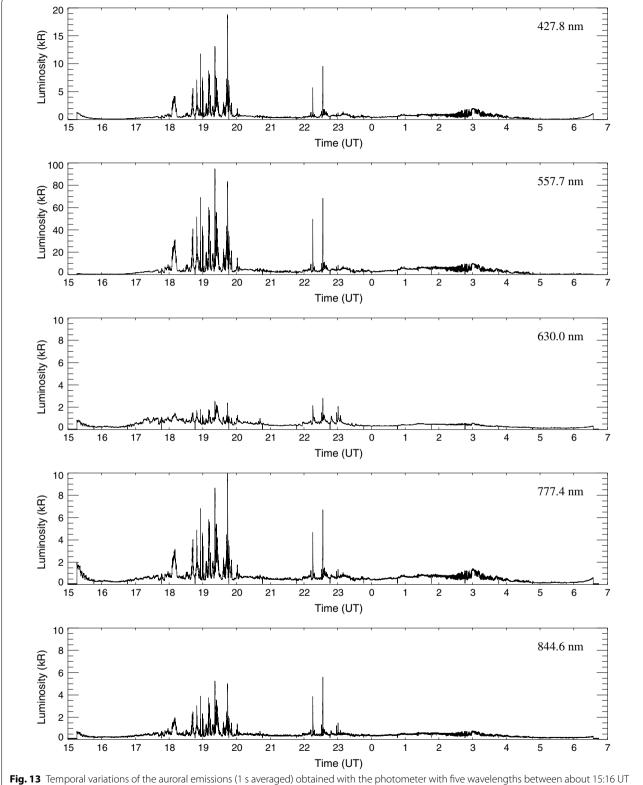
Fig. 13 lemporal variations of the auroral emissions (1 s averaged) obtained with the photometer with five wavelengths between about 15:16 UI on January 22, 2018, and about 06:35 UT on January 23, 2018. The emissions of 427.8 nm, 557.7 nm, 630 nm, 777.4 nm, and 844.6 nm (1 s averaged data) are presented from top to bottom
