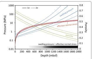
**Fig. 4** Porosity and swelling pressure curves at depths of the fault zone. Swelling pressure (blue), effective normal stress (red) and porosity (green) at depths of the fault zone extrapolated from the porosity-depth and porosity-swelling pressure curves (Figs. 1b and 3)
