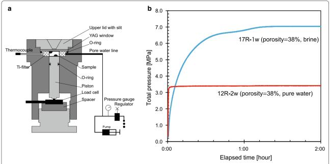
Fig. 2 Apparatus and typical results of the swelling pressure tests. a Schematic diagram of the test apparatus used in this study. b Typical swelling pressure measurements for the fault zone sample (blue line) and the host rock sample (red line). Note that the fluid pressure was fixed at 0.2 MPa
