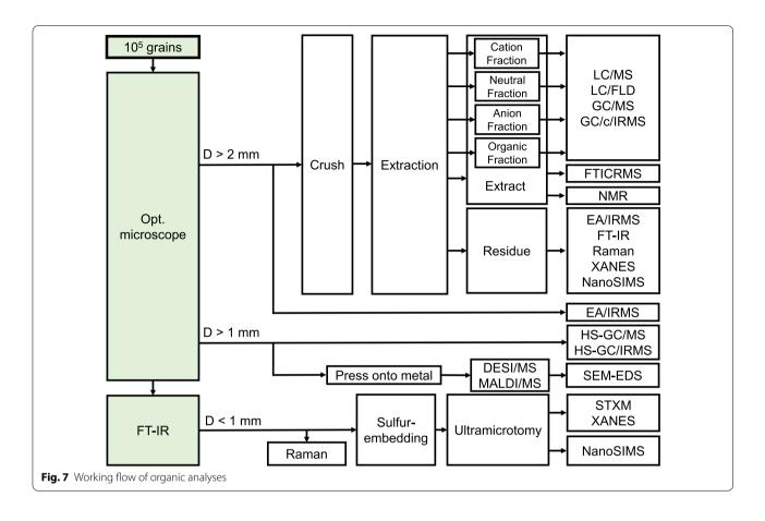
baseline resolution of target molecules and high amounts of specifically interested extractable organic compounds (e.g., amino acids and sugars), their compound-specific C and N isotope compositions will be analyzed with gas chromatography/combustion/isotope ratio mass spectrometry (GC/C/IRMS) (e.g., Aponte et al. 2014; Elsila et al. 2016b; Chan et al. 2016; Glavin et al. 2018; Furukawa et al. 2019).
