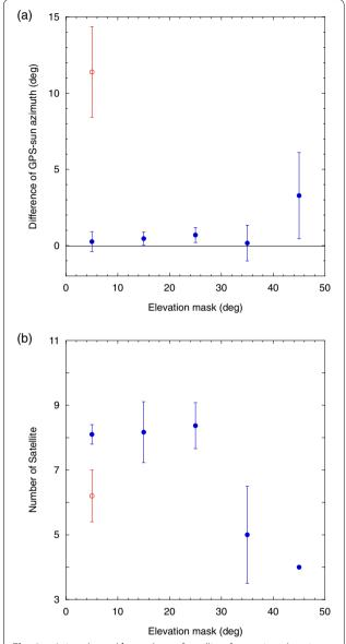
**Fig. 4** a Azimuths and **b** numbers of satellites for varying elevation mask at a site with open sky (blue) and a site between buildings (red). The root-mean-squares are indicated by vertical bars. For 45°, the number of satellites was constant at four
