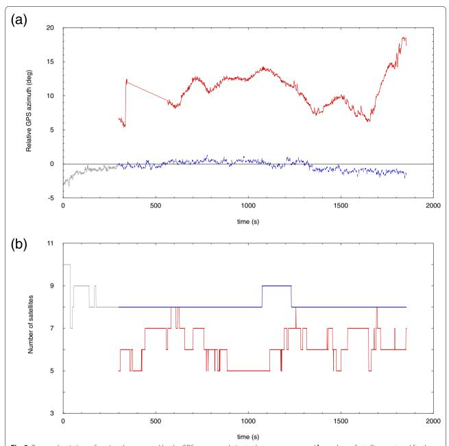
**Fig. 2** Temporal variations of **a** azimuths measured by the GPS compass relative to the sun compass and **b** numbers of satellites captured for the GPS signals, at a site with open sky (blue) and a site between buildings (red). The first 5 min at the open site, shown in gray, did not give reliable azimuths due to initialization of the GPS compass. At the site between the buildings, data were not collected during the first 5 min
