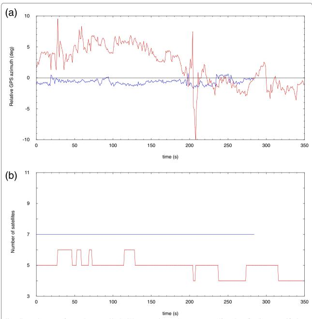
**Fig. 5** Temporal variations of **a** azimuths measured by the GPS compass relative to the sun compass and **b** numbers of satellites captured for the GPS signals for drill cores at coast and forest sites. Blue indicates data at a coast site (site 28, core 250) where the sky above is open, red indicates data at a forest site (site 31, core 114) where the vertical outcrop is covered by trees. At both sites data were not recorded during the first 5 min for initialization of GPS compass
