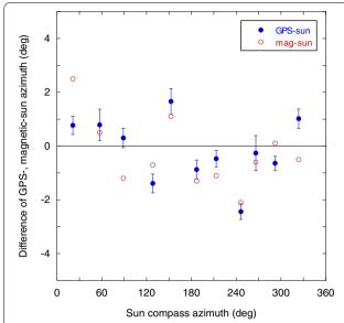
**Fig. 3** Azimuths measured by the GPS and magnetic (mag) compasses relative to the sun compass for 11 different directions. At the measurement site the sky above is open and the elevation mask was set to 5°. For the GPS compass, azimuthal data were acquired for about 30 min at 1 Hz, and the root-mean-squares are indicated by vertical bars
