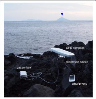
**Fig. 1** A portable GPS compass mounted on an orientation device of a paleomagnetic drill core. A battery box supplies DC 12 volts by ten AA rechargeable batteries through a wire, and a smartphone acquires the GPS data through Bluetooth wireless connection. An arrow points to the landmark for backsighting
