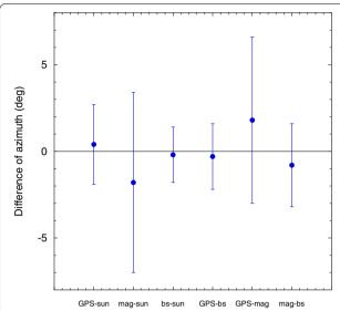
**Fig. 6** Differences of azimuths measured by the sun, GPS, and magnetic (mag) compasses and backsighting (bs) for drill cores. The root-mean-squares are indicated by vertical bars
