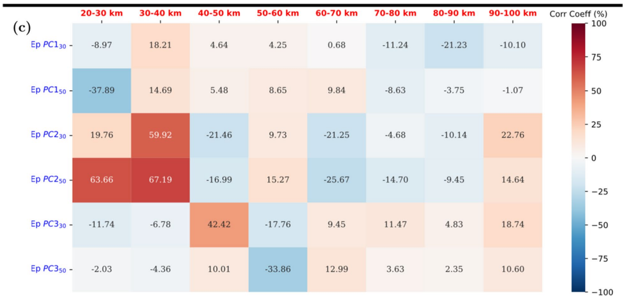
Fig. 8 The temporal variation of the EOF2 at 30–40 km (a) and 20–30 km (b) over the 20-year period, and the QBO measurement at 30 mb (solid line in magenta) and at 50 mb (dotted line in red). c is the correlation coefficients (in %) of the Ep and QBO at 30 mb and 50 mb
