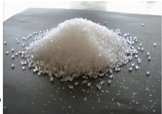
Fig. 2. Left: Transmission rate of the present plastic scintillator sample (length 12 cm). Right: The produced pellet polymer.
