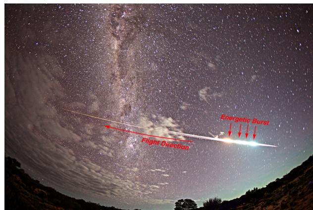
Fig. 2. A long exposure photograph of the Hayabusa reentry fireball. Canon EOS 5D mark II with 15 mm diagonal fisheye, F/2.8, ISO = 3200, and a 120-s exposure.
