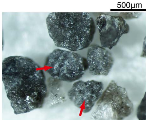
Fig. 8. Lava particles in April 3, 2011 ash (250–500 \mu\text{m} fraction) which were classified into “fresh lava” because of similar appearance to “fresh lava” particles in February to March vulcanian ash samples (e.g. Figs. 7(a)–(b)). However, “fresh lava” particles in April 3 ash are partly altered (red arrows). The photograph was taken under binocular microscope. For definition of lava particles and its sub-types (“fresh” and “partly-altered”), see Subsection 5.1.1. Color version available online.
