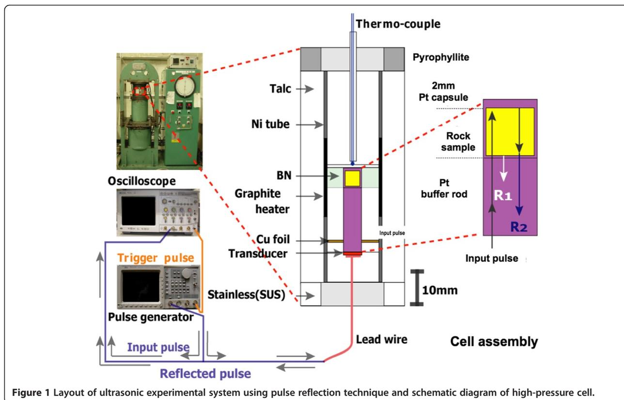
City, Japan). Talc, pyrophyllite, and boron nitride (BN) were used as the solid pressure transmitting medium that also contained a heating element and sample. The calibration of pressure has been described elsewhere (Kono et al. 2004, 2008; Kozai and Arima 2005; Nishimoto et al. 2005).
