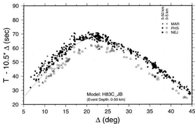
Fig. 5. Picked travel times of the first arrivals. Circles, diamonds, and triangles represent data from NEJ, PHS, and MAR data set, respectively; open and filled symbols are of shallow ( $d = 0-5$  km) and deep ( $d = 5-50$  km), respectively. Solid line indicates  $P$  arrival times for the standard time table of Hamada (1984). Note that there is an offset of approximately 5 seconds for some data points, all of which are of shallow ( $0-5$  km) events.
