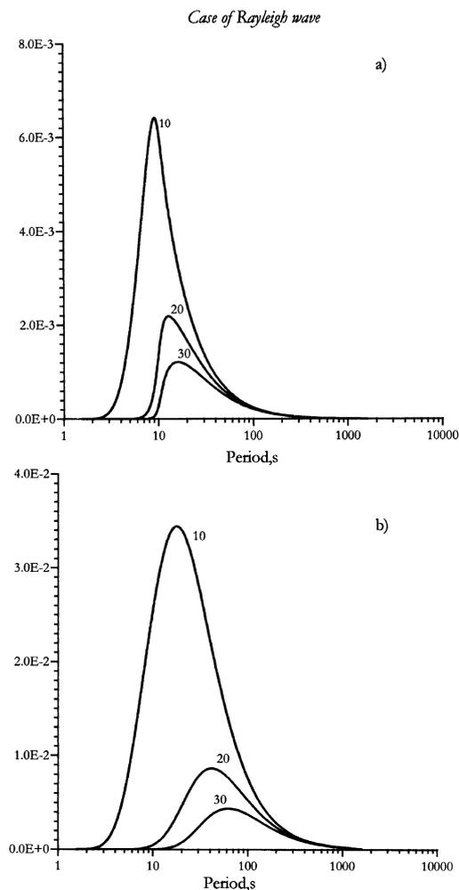
Fig. 6. The dependence of  $|q(h, \omega, \varphi)|$  on period for the dip-slip source located a) in gravitating half space model III, b) in gravitating half-space model I. Results without gravitational force are identical. Numbers at the curves indicate the source depth in half-space.
