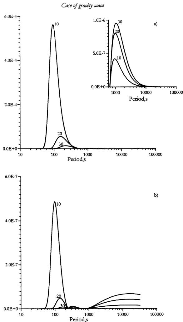
Fig. 2. The dependence of  $|q(h, \omega, \varphi)|$  with period for dip-slip source located a) in non-gravitating half-space, b) in gravitating half-space. Numbers at the curves indicate the source depth in half-space.
