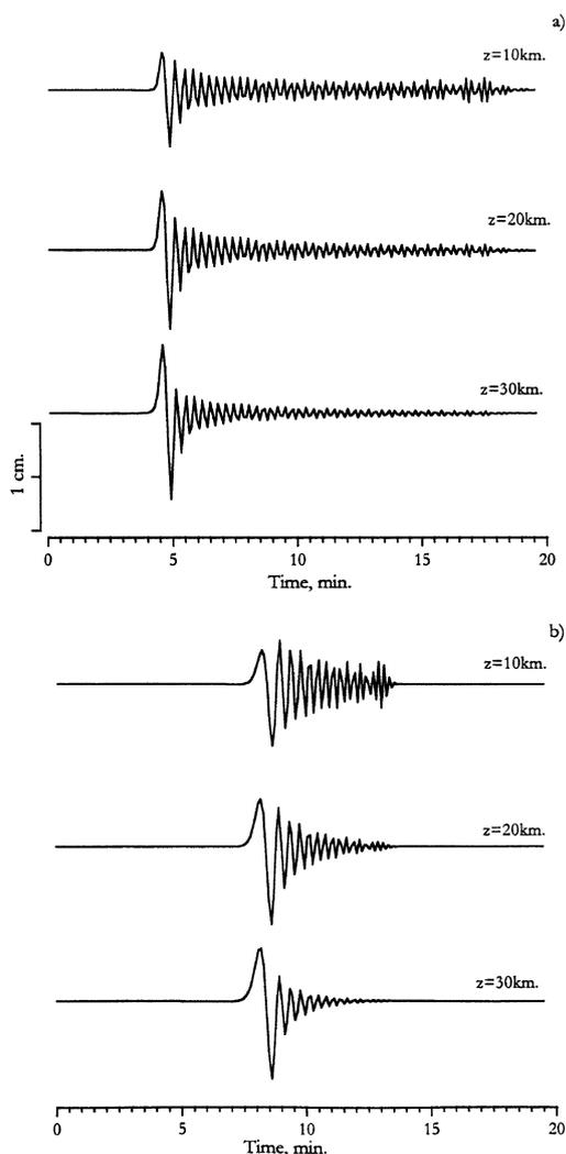
Fig. 7. A comparison of theoretical marigrams of Rayleigh wave from the dip-slip source a) for model III, b) for model II with gravitating half-space. Results without gravitational force are identical. The right numbers at the curves indicate the source depth in half-space.
