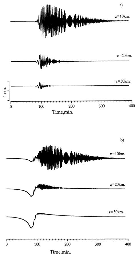
Fig. 5. A comparison of theoretical marigrams of gravity wave from the dip-slip source for model III a)- with non-gravitating half-space, b)- with gravitating half-space. The right numbers at the curves indicate the source depth in half-space.
