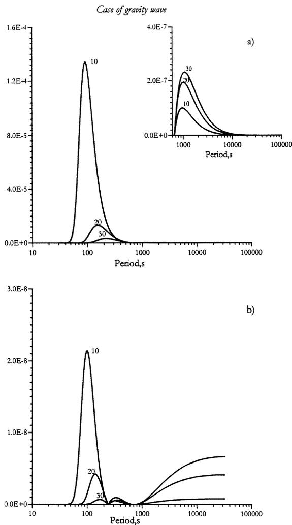
Fig. 3. The dependence of  $|q(h, \omega, \varphi)|$  with period for dip-slip source located a) in non-gravitating half-space, b) in gravitating half-space. Numbers at the curves indicate the source depth in half-space.
