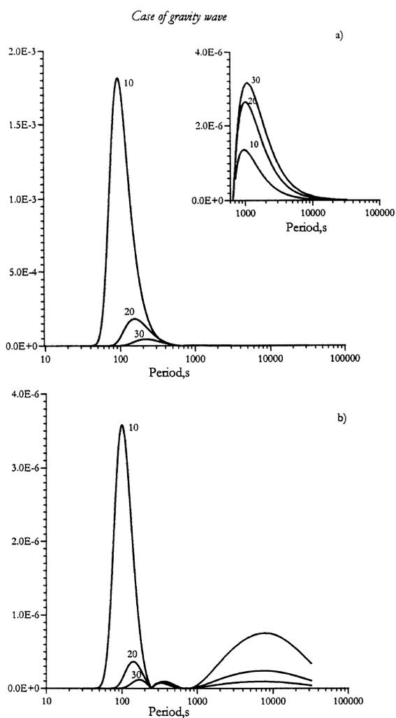
Fig. 1. The dependence of  $|q(h, \omega, \varphi)|$  on period for the dip-slip source located a) in non-gravitating half-space, b) in gravitating half-space. Numbers at the curves indicate the source depth in half-space.
