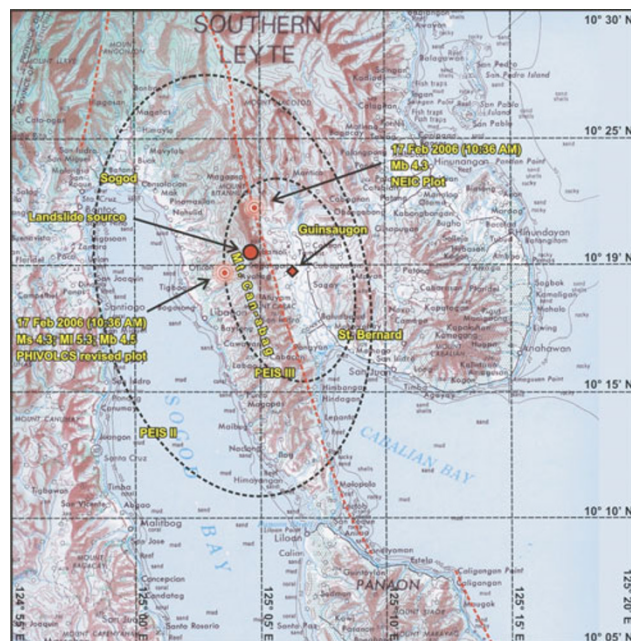
Fig. 2. Earthquake location and intensity map. The Philippine Institute of Volcanology and Seismology (PHIVOLCS) Earthquake Intensity Scale (PEIS) score was based on field interviews of residents in St. Bernard and adjacent municipalities as far as Sogod. The uninhabited and inaccessible northwest quadrant of the isoseismal map was inferred (modified from Daag et al. , 2006).
