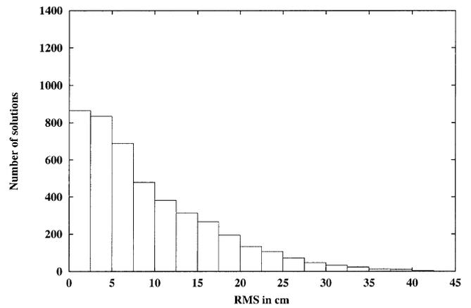
Fig. 9. Histogram of RMS of GPS/MET phase position differences using 10-second data and quadratic satellite clock interpolation.
