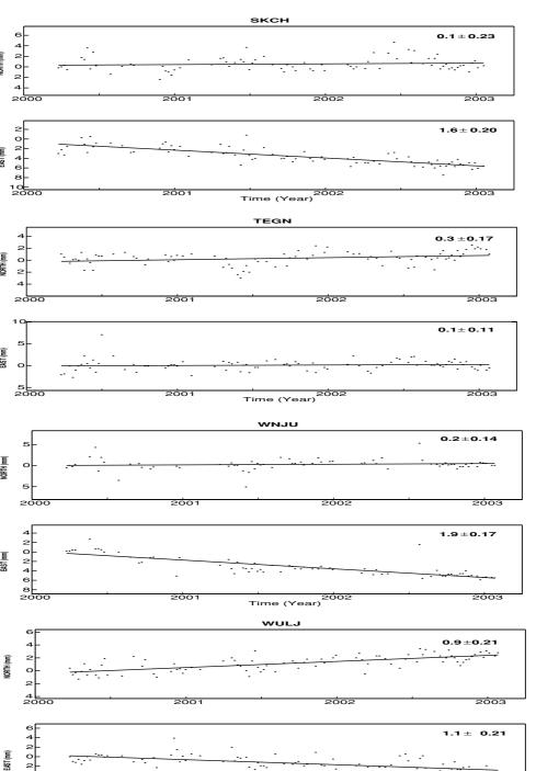
Fig. 3. Time series of horizontal coordinates for some selected sites with respect to the DAEJ station. Solid lines are the best fit lines for temporal changes of the east and north components.
