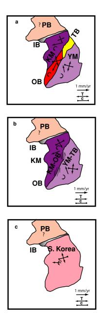
Fig. 4. Deformation of South Korean blocks (2000–2003). A, B and C show cases assuming 4, 2 and 1 blocks, respectively. Arrows are not to scale (for the values see table 1). Abbreviations are the same as in Fig. 2.
