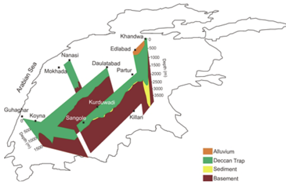
Fig. 6. Fence diagram showing the variation of trap thickness along all the five traverses across the DVP.
