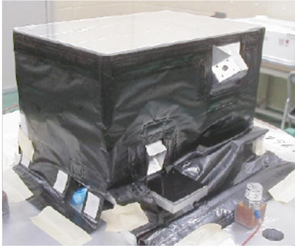
Fig. 2. Photograph of the Solar Monitor (SOL-BC) is shown. A Si-PIN diode based solar X-ray direct monitor (SOL-B) at the upper right position of the SOL-BC and a CCD-based XRF calibrator with a fused sample plate (SOL-C) at the lower center position are united as a single component. The top side is a radiator. SOL-BC is mounted to the top panel of SELENE.
