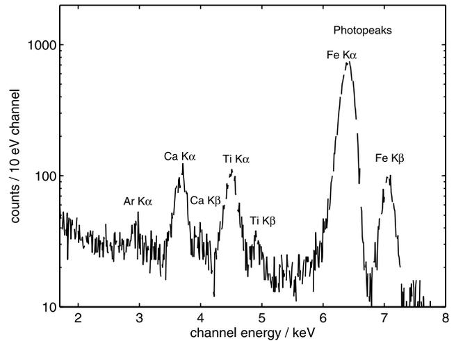
Fig. 3. A typical x-ray spectra as function of photon energy obtained by XRF-A at  $-40^{\circ}\text{C}$ . The specimen used here is also a glassy plate as the one equipped for SOL-C (Table 2), except that Mn, Cr, K, Na are not included as its composition. The spectrum shows photopeaks for Fe, Ti, Ca, and Ar. Ar photopeak is detected in absent of expected peaks for Mg, Al, and Si due to attenuation of low energy x-ray in the air.
