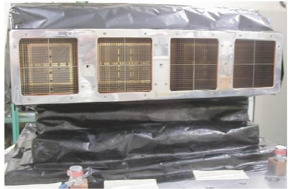
Fig. 1. Photograph of the Lunar X-ray fluorescence detector (XRF-A) is shown, viewed from the side of the latticed collimator for 16 CCD chips. Beryllium light-tight window can be seen inside. Backside of CCD chips is thermally connected to a radiator, not seen in this figure. XRF-A is mounted on the side panel of SELENE, detector facing to the lunar surface.
