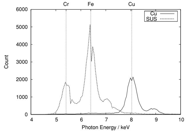
Fig. 5. The x-ray spectra as a function of photon energy obtained by SOL-B at  $0^{\circ}\text{C}$ . The specimen used here are steel plate (SUS) and copper plate.
