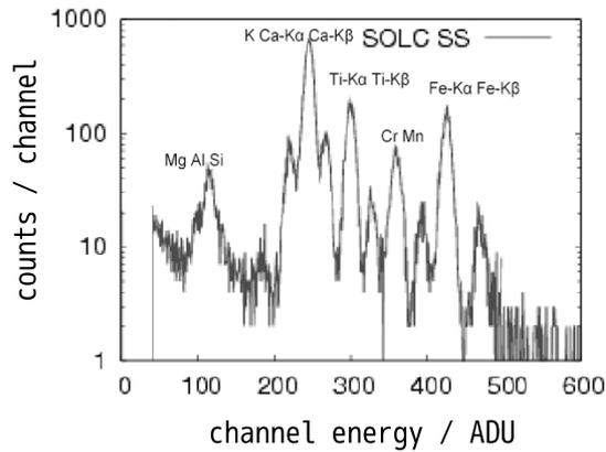
Fig. 4. A typical x-ray spectra as function of photon energy obtained by SOL-C at  $-40^{\circ}\text{C}$ . The specimen used here is a glassy plate equipped for SOL-C (Table 2). The spectrum shows photopeaks for Mg, Si, K, Ca, Ti, Cr, Mn, Fe. The experiment is performed in vacuum condition.
