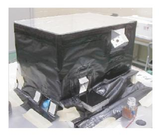
Fig. 2. Photograph of the Solar Monitor (SOL-BC) is shown. A Si-PIN diode based solar X-ray direct monitor (SOL-B) at the upper right position of the SOL-BC and a CCD-based XRF calibrator with a fused sample plate (SOL-C) at the lower center position are united as a single component. The top side is a radiator. SOL-BC is mounted to the top panel of SELENE.
