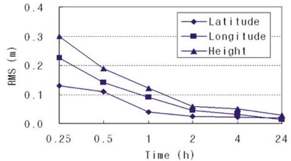
Fig. 2. Expected positioning accuracy of CSRS-PPP as a function of time (Geodetic Survey Division).
