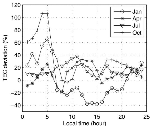
Fig. 6. Monthly averaged diurnal TEC variation percentage of GPS reconstruction with respect to the IRI-2001 model.
