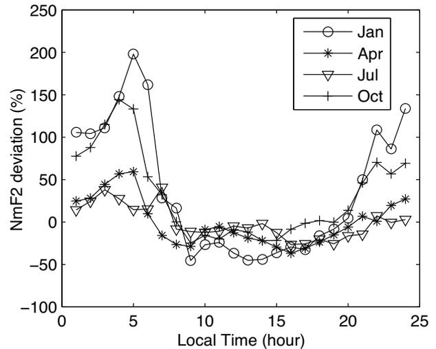
Fig. 4. Monthly averaged diurnal NmF2 variation percentage of the GPS reconstruction with respect to the IRI-2001 model.
