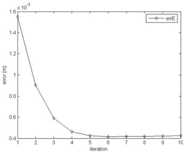
Fig. 4. Error versus iteration for the simulated network with 1 million points.
