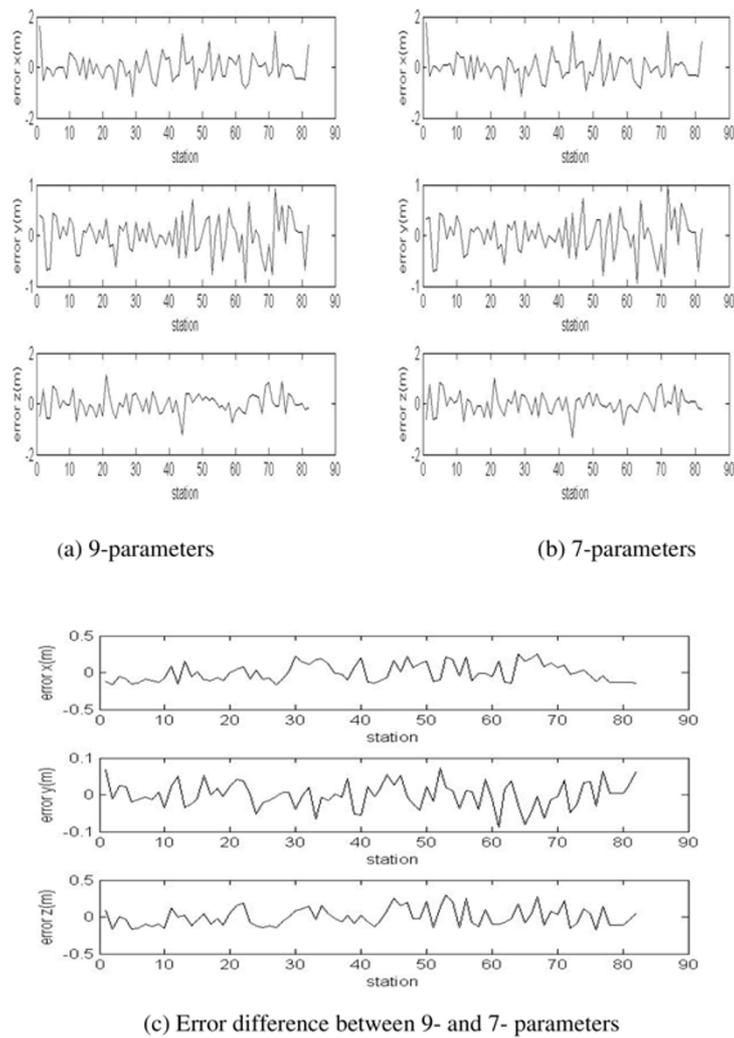
Fig. 6. Error plots of each station for 82 stations in WA, Australia (AGD84 and GDA94) with 9- and 7-parameters.
