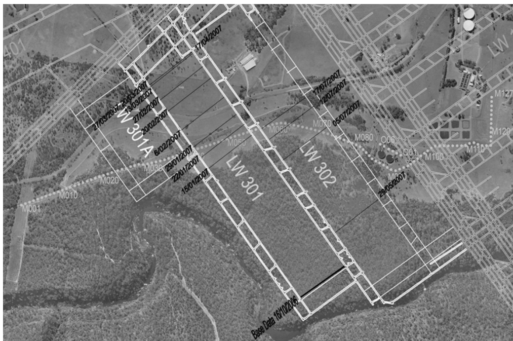
Fig. 12. Appin Mine Site (with longwall structure overlaid on an aerial photo). (©BHP Billiton)
