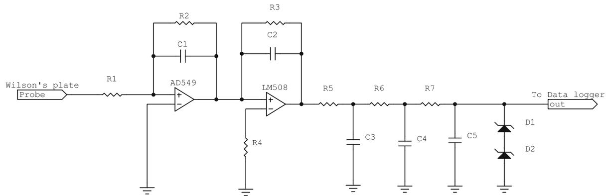
Fig. 1. Circuit diagram of the Wilson's plate experiment.
