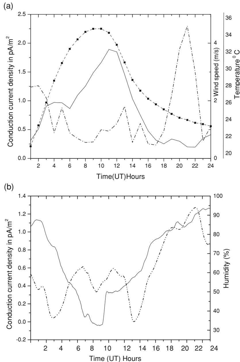
Fig. 2. (a) The variation air-earth current with temperature and wind speed of the troposphere on a fair-weather day, the dotted line represent conduction current, the dashed line plus simple line shows the temperature and the continuous line shows wind speed. (b) Variation in conduction current with local humidity. The dotted line represents the conduction current and the continuous line, the humidity.
