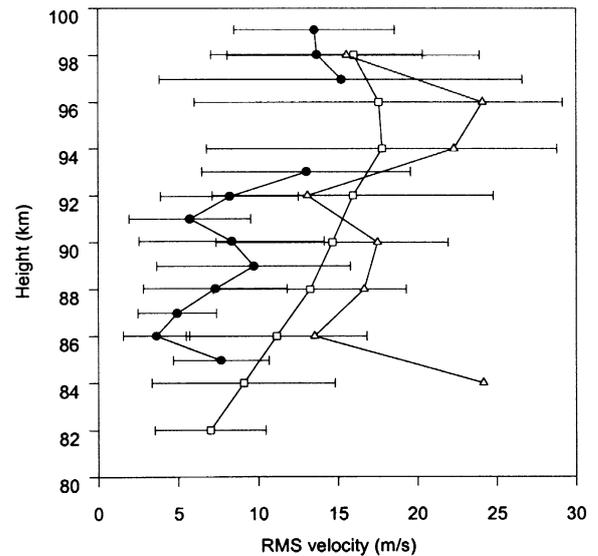
Fig. 2. Comparison of RMS velocity measurements between an Na lidar and an MF radar. Solid circles with 95% confidence bars denote the lidar measurements, squares with 90% confidence bars denote the one-day average measurements by MF radar, and triangles denote the 11–14UT average measurements by MF radar.
