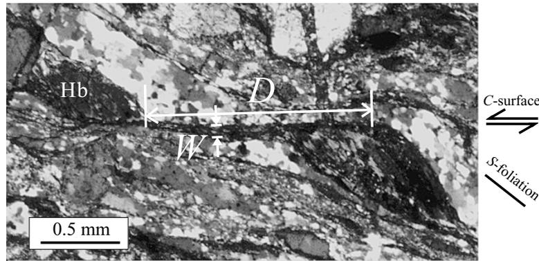
Fig. 3. Thin section of a shear displaced mineral (hornblende: Hb) along  $C$ -surface in S-C mylonite. Displacement ( $D$ ) is measured from a distance between each mineral, showing a same orientation of cleavage planes. Width ( $W$ ) is measured as a localized sheared zone along  $C$ -surface (black arrows), cutting obviously through mylonitic  $S$ -foliation (black bar).
