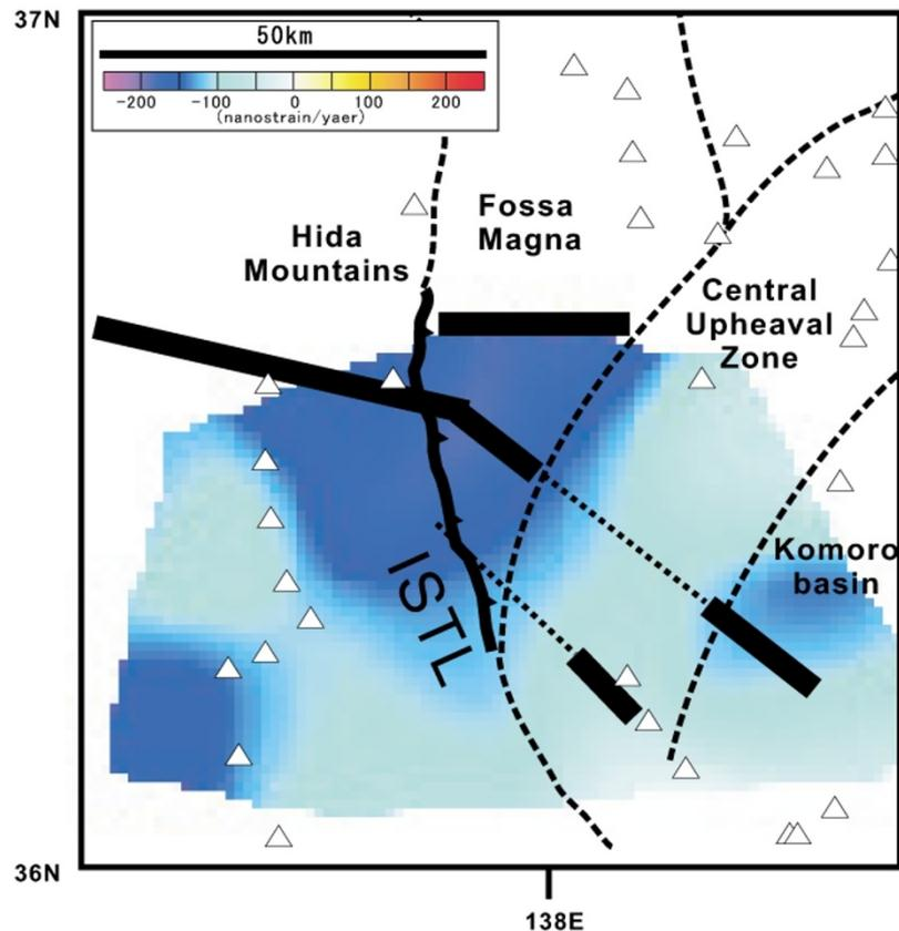
Fig. 4. Distribution of the mid-crustal conductors and the dilatation anomaly (Sagiya *et al.*, 2004). MT profiles are shown by lines and the locations of the mid crustal conductors are shown by bold lines.
