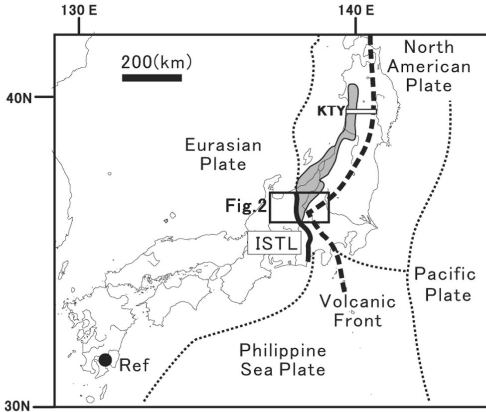
Fig. 1. Location of the study area in the central Japan in the framework of plate configurations. ISTL is shown as a thick line in Central Japan, which is regarded as a boundary between North-American and Eurasian Plates. Ref shows the location of the remote reference site for magnetotelluric measurements. The gray area along the Japan Sea coast is the thick Miocene sedimentary basin created by the Japan Sea opening. KTY is another MT profile by Ogawa *et al.* (2001).
