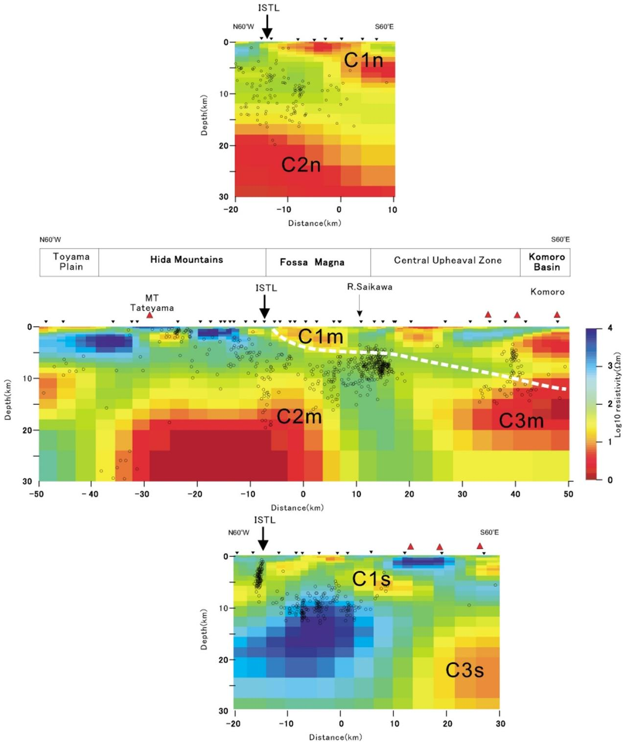
Fig. 3. Two-dimensional models for the north, the main and the south profiles. Major conductors are labeled. The triangles denote approximate locations of the nearby Quaternary volcanoes. The estimated fault geometry was plotted on the main profile with white line. The hypocenters were also projected using JMA dataset (from 1997 to 2002) along the profile with 10 km width.
