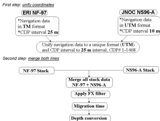
Fig. 2. Processing sequence of the merged line (NF-97 and NS96-A).
