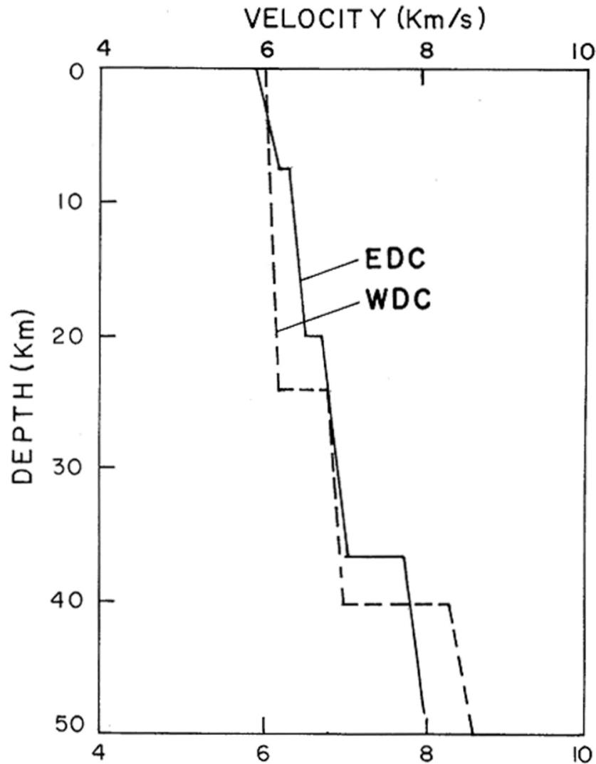
Fig. 5. Crustal  $P$ -wave velocity-depth distribution for WDC and EDC (after Reddy *et al.*, 2000).
