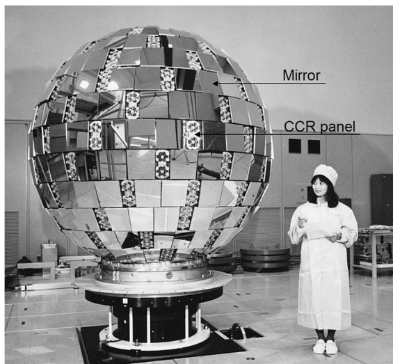
Figure 1 Ajisai (courtesy of JAXA) and positions of the CCR panels on the surface. The retroreflector array consists of 15 rings R_{-7} \dots R_7 ; R_0 is the equator ring.
