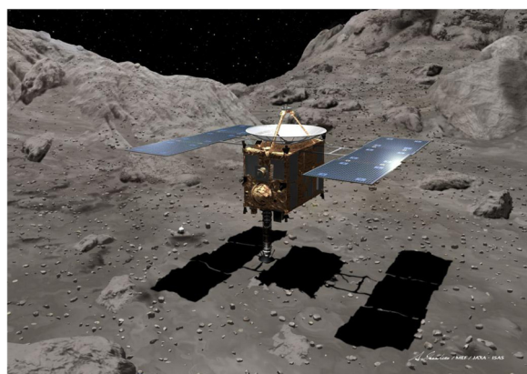
Fig. 2 An artist view of the Hayabusa spacecraft just a moment before the touchdown on the surface of asteroid 25143 Itokawa for sampling with the horn-shaped sampler (Ikeshita/MEF/JAXA-ISAS). Actual result was that the impact sampler failed to shoot the projectile for excavating the surface materials and collecting part of them into the sample catcher, but only the dusts floating around there were obtained and consequently returned to Earth
