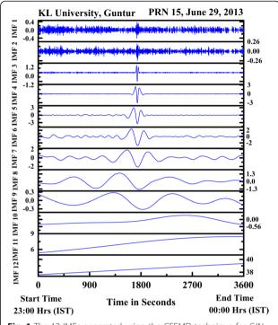
**Fig. 1** The 12 IMFs generated using the CEEMD technique for  $C/N_0$  values of PRN 15 on 29 June 2013 sampled at 1 Hz rate
