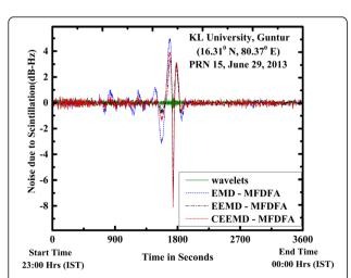
${\bf Fig.~3}$  The results of the CEEMD–MF-DFA method in reducing the noise from the GPS signal
