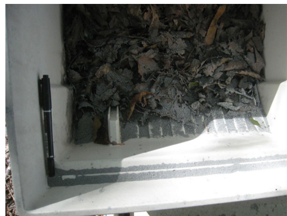
Fig. 3 Photograph of the sampling point of pyroclastic material OT-3, a roadside garbage box, in the morning of September 30, 2014
