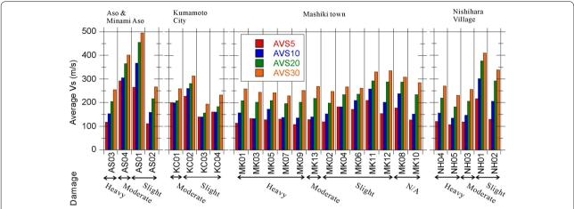
Fig. 5 Average S-wave velocities in the upper 5, 10, 20, and 30 m evaluated from the detailed S-wave velocity profiles with the degree of damage for each site reported by Yamanaka et al. (2016)
