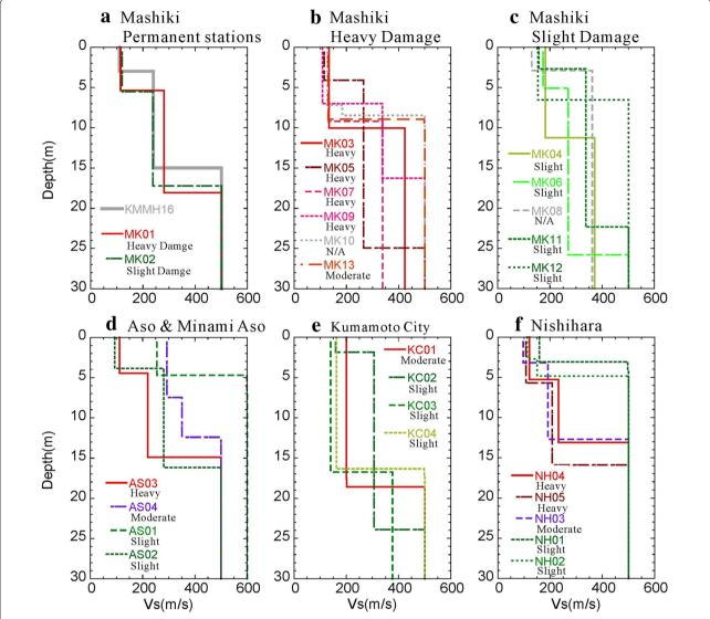
Fig. 4 S-wave velocity profiles estimated from the inversion of the phase velocity in Mashiki (a-c), Aso and Minamiaso (d), Kumamoto (e) and Nishihara (f). The line labeled "KMMH16" represents the results for the model obtained from the borehole logs at the station KMMH16
