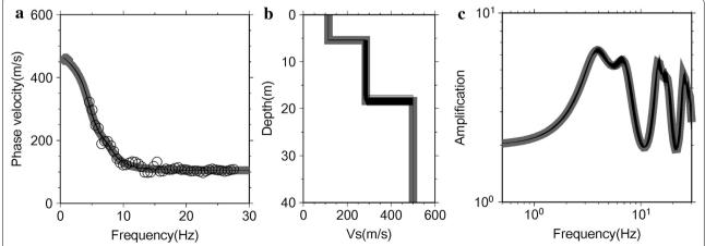
**Fig. 3** a Observed phase velocity at MK01 (*circles*) and the calculated phase velocity curve for the best-fit model (*gray line*). The curves that differ from the best-fit curve by a maximum of 1% (acceptable curves) are shown as *thin solid lines*. **b**  $V_S$  profiles for the best-fit phase velocity curve (*gray*) and acceptable curves (*thin solid line*). **c** Amplification for the best-fit model (*gray*) and acceptable models (*thin solid line*)
