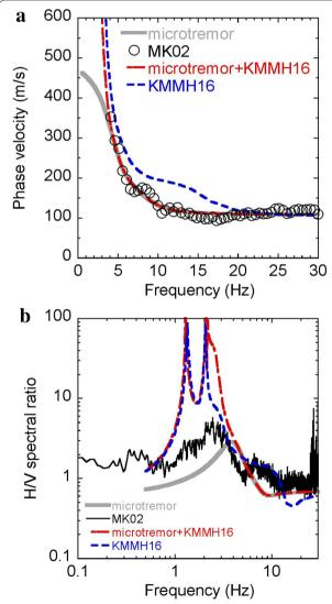
**Fig. 9** a Comparison of observed phase velocity curves (*circles*) with those calculated for the model at KMMH16 (*blue*), for the shallow  $V_S$  model determined from the observed microtremors (*gray*), and for the replacement  $V_S$  model in the shallow part of the  $V_S$  structure determined from the observed microtremors (*red*). **b** Same comparison as in (**a**) for the H/V
