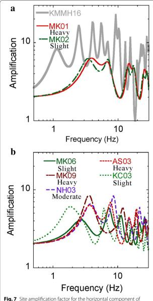
**Fig. 7** Site amplification factor for the horizontal component of S-waves assuming one-dimensional vertically incident propagation from the engineering bedrock at two permanent station sites (**a**) and other sites (**b**). The *gray line* in (*a*) shows the computed results for the model at KMMH16
