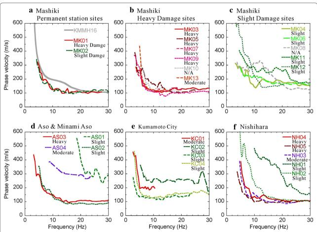
**Fig. 2** Phase velocity dispersion curves in Mashiki (**a–c**), Aso and Minamiaso (**d**), Kumamoto (**e**) and Nishihara (**f**). The *gray line* in (**a**) shows the calculation results for the model obtained at KMMH16 from borehole logs. In each plot, *warm* and *cool colors* correspond to sites experiencing heavy and light damage, respectively
