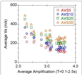
**Fig. 8** Average S-wave velocity in the top 5, 10, 20, and 30 m plotted against the amplification averaged over the period range of 0.1–2.5 s
