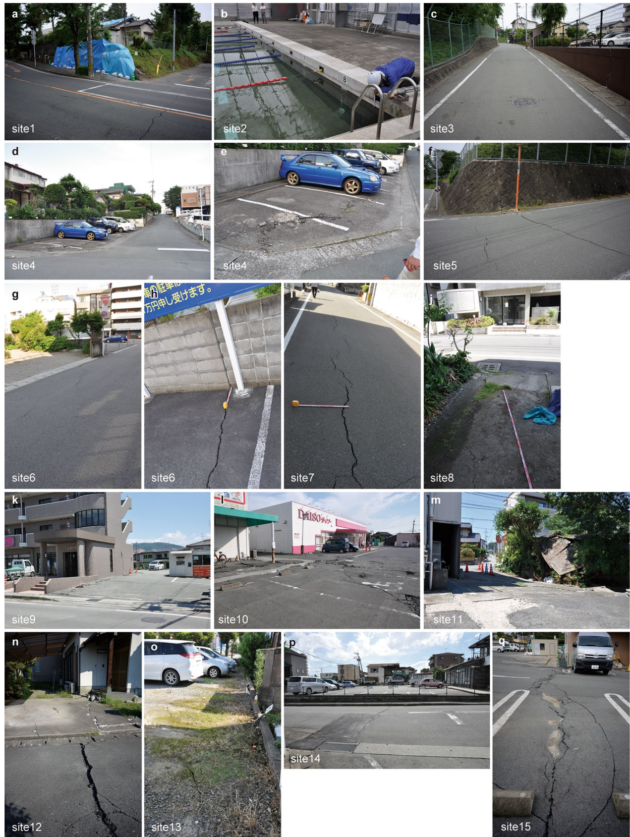
Fig. 7 Snapshots of surface deformation along the Suizenji fault zone ( site 1–8 ) and the Akitsukawa flexure zone ( site 9–15 ). The localities of the site are shown in Fig. 3
