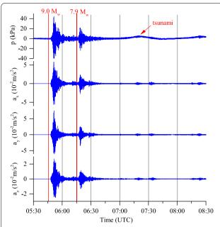
**Fig. 2** Pressure (p) variations and acceleration components  $a_x$ ,  $a_y$  and  $a_z$  registered by DONET observatory A02 on March 11, 2011. The red vertical lines indicate the time of the main shock and of the first strong aftershock
