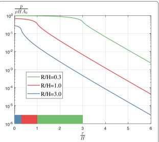
**Fig. 5** Dependence of amplitude of pressure variations at ocean bottom, caused by a round source (vertical oscillations of a segment of the ocean bottom), upon the distance from the source center. The calculation is done for three different source sizes (indicated in the figure). The size and shape of the sources are shown in the left bottom corner as rectangles of the corresponding color
