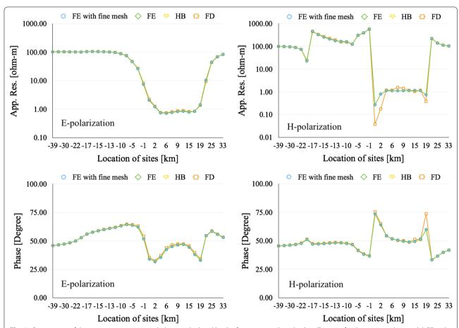
**Fig. 9** Comparison of the apparent resistivity and phases calculated by the four numerical methods at  $T=10\,\mathrm{s}$  for the topographic model: FE with fine mesh (circle), FE (diamond), HB (triangle) and FD (square) methods. The apparent resistivities for the *E*- and *H*-polarizations are at the left and right top, respectively, whereas the phases for the *E*- and *H*-polarizations are at the left and right bottom, respectively
