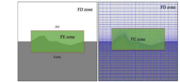
**Fig. 3** The model with setting of the FD and FE zones (left). The FE zone is set and optimized for the terrain zone (light green), whereas the FD zone is set for the simple zone without terrain. Design of the mesh of the FD and FE zones (right). Quadrilateral elements are used for the FE zone, whereas rectangular blocks are used for the FD zone
