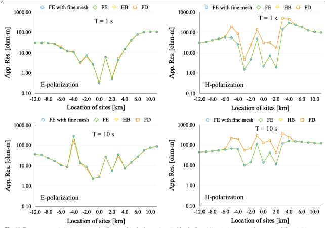
**Fig. 12** The apparent resistivities computed at T=1 s of the bathymetric model for the E- and H- polarizations are shown at the left and right top, respectively, whereas those computed at T=10 s are shown at the left and right bottom, respectively
