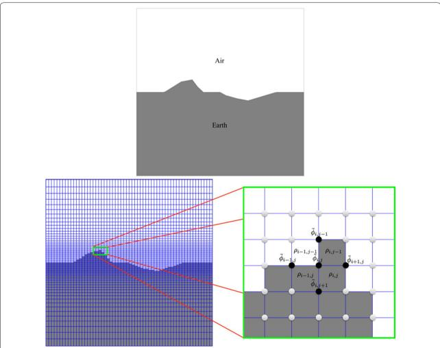
**Fig. 1** The resistivity model with terrain (top). The discrete model with rectangular blocks (left bottom). The approximation of field  $\tilde{\phi}$  by using the four neighbor nodes is demonstrated (right bottom)
