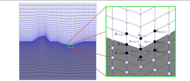
**Fig. 2** The discretized model with quadrilateral elements (left). The approximation of field  $\tilde{\phi}$  by using the eight neighbor nodes is demonstrated (right)
