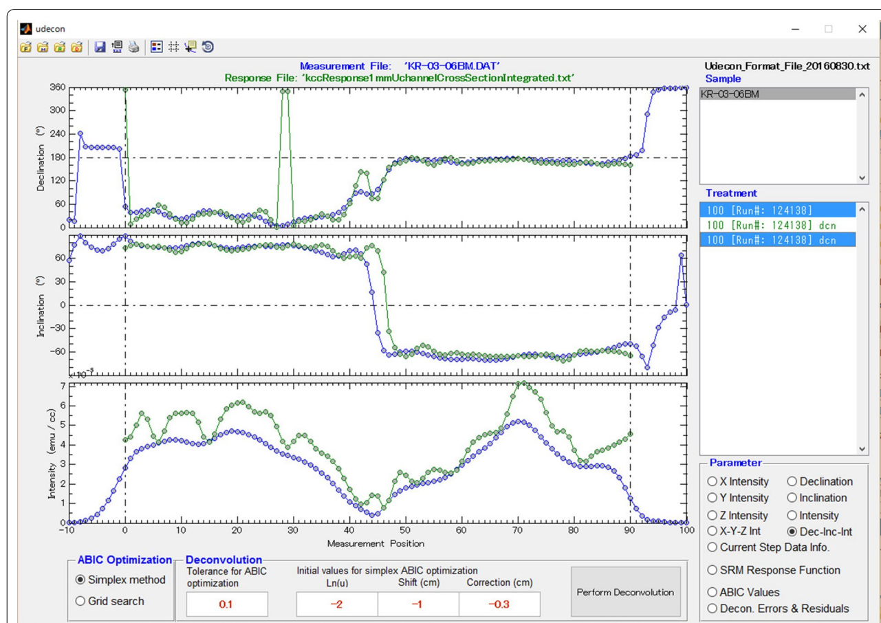
Fig. 3 Screen shot of results obtained by the software UDECON. Data points connected by blue lines are from the u-channel sample, and those connected by green lines are deconvolved data. The deconvolved data were obtained by using the three parameter values in the lowermost panel as initial input values
