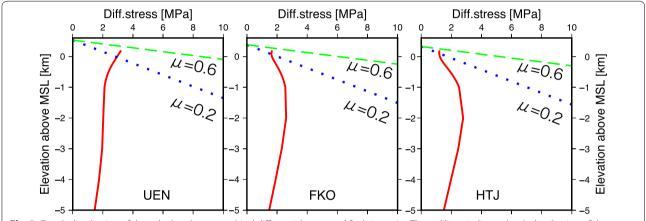
**Fig. 3** Depth distribution of the calculated topographical differential stress and fault intensity. The red lines indicate depth distribution of the differential stress. The blue dotted and green dashed lines denote fault strength ( $= \mu \rho q z$ ) with a friction coefficient  $\mu = 0.2$  and 0.6, respectively
