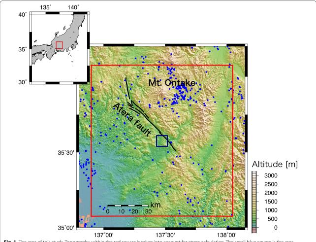
**Fig. 1** The area of this study. Topography within the red square is taken into account for stress calculation. The small blue square is the area shown Fig. 2. The blue small circles denote shallow seismicity (2001–2010) with magnitude of > 1 and a depth of < 20 km around the Atera Fault determined by Japan Meteorological Agency. The black lines denote the Atera Fault
