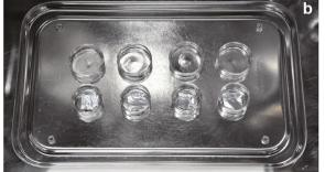
**Fig. 1** a The clean chamber in the curation room at ISAS/JAXA and **b** the witness coupons placed in the chamber
