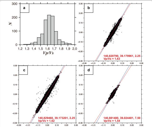
**Fig. 6** a Histogram of  $V_p/V_s$  ratios estimated in this study and **b-d** examples of the data distributions. Slope of the red line represents the local  $V_p/V_s$  ratio for the cluster. Blue line is drawn as a reference whose slope is 1.73. Red texts represent the center of the longitude, latitude and depth ranges, and  $V_p/V_s$  ratio for the corresponding data
