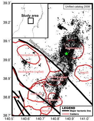
**Fig. 1** Distribution of calderas, tectonic lines, and earthquakes in the study area. Calderas and tectonic lines are from Nunohara et al. (2010) and Baba (2017), respectively. Epicenters of earthquakes in 2008 at depths ≤ 15 km are shown as black dots and are from the JMA unified catalog. The green star denotes the mainshock epicenter estimated by Okada et al. (2012)
